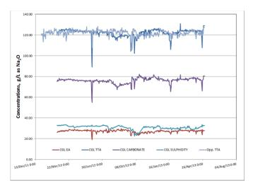
Figure 4. Trend of CGL data from analyzer since Feb. 2012. An overlay of the manual operations TTA value show good correlation.
