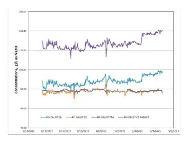
Figure 5: 4<sup>th</sup> Causticizer EA, TTA, and CE trend. 4<sup>th</sup> Causticizer CE target tracks well with FT-NIR CEs.
