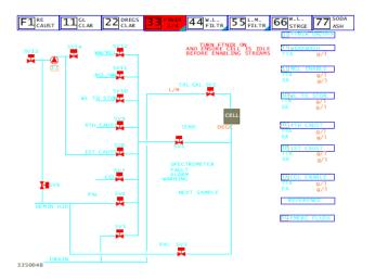
Figure 2: DCS schematic of the analyzer piping and valve operations.
